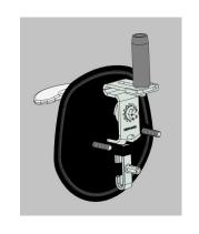
Slide in BOLT that has the post into HANDLE BODY.
