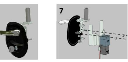
Install WHALE-T HANDLE into application from the front, mount the EM POWER MODULE BRACKET ASSEMBLY from the inside of the application with the NUTS.
