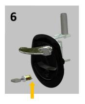
With the KEY inserted in KEY CYLINDER, install the KEY CYLINDER into the HANDLE BODY from the front, while inserting make sure to align PIN on back of CYLINDER and depress RETAINING RING on KEY CYLINER, insert until Cylinder is flush to face of Handle.
