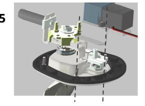
Install EM POWER MODULE BRACKET ASSEMBLY, aligning the POWER MODULE PIN to the BOLT, and position bracket over LOWER STUDS
