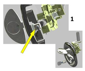
To REMOVE the KEY CYLINDER, Depress RETAINING RING thru the HOLE in the BARREL and pull out KEY CYLINDER using the KEY inserted in KEY CYLINDER
