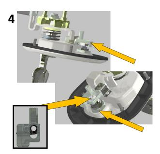
Stack the BOLT on top of CAM (see alignment) position on LOCK ASSEMBLY using the BUTTON HEAD SCREW tighten fully.
