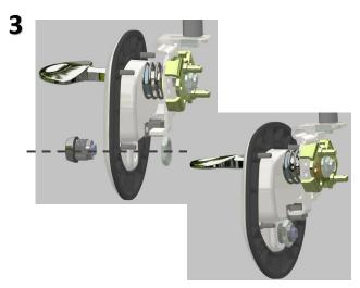
Insert NEW LOCK ASSEMBLY into hole, and thread NUT partial on
