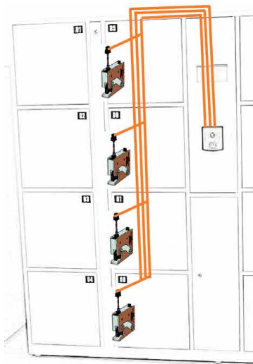
OPTION 1 5-Wire Activation with Feedback Sensor Power +/-, Activation Signal Feedback Sensor NO/C
