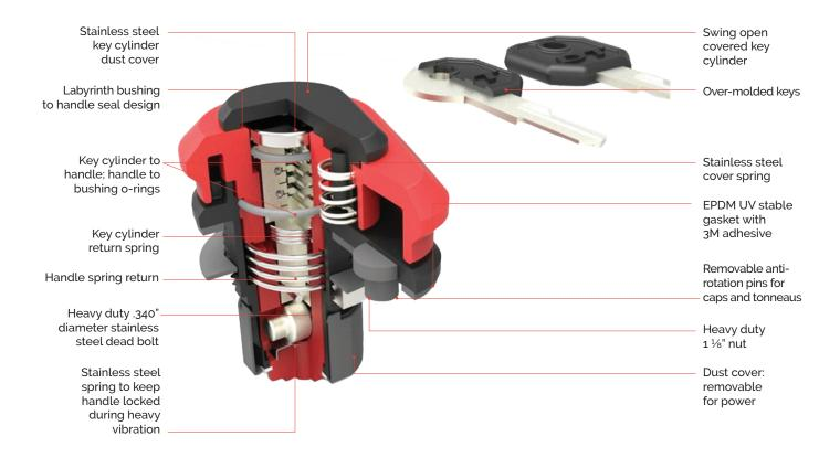
Our mechanical handles are designed and built to be power adaptable. The module can be installed by the OEM or as an aftermarket addition.
